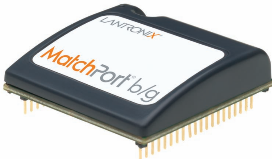
Figure 2 | The MatchPort b/g provides an easy way to integrate an 802.11b/g link onto the main CPU board.
