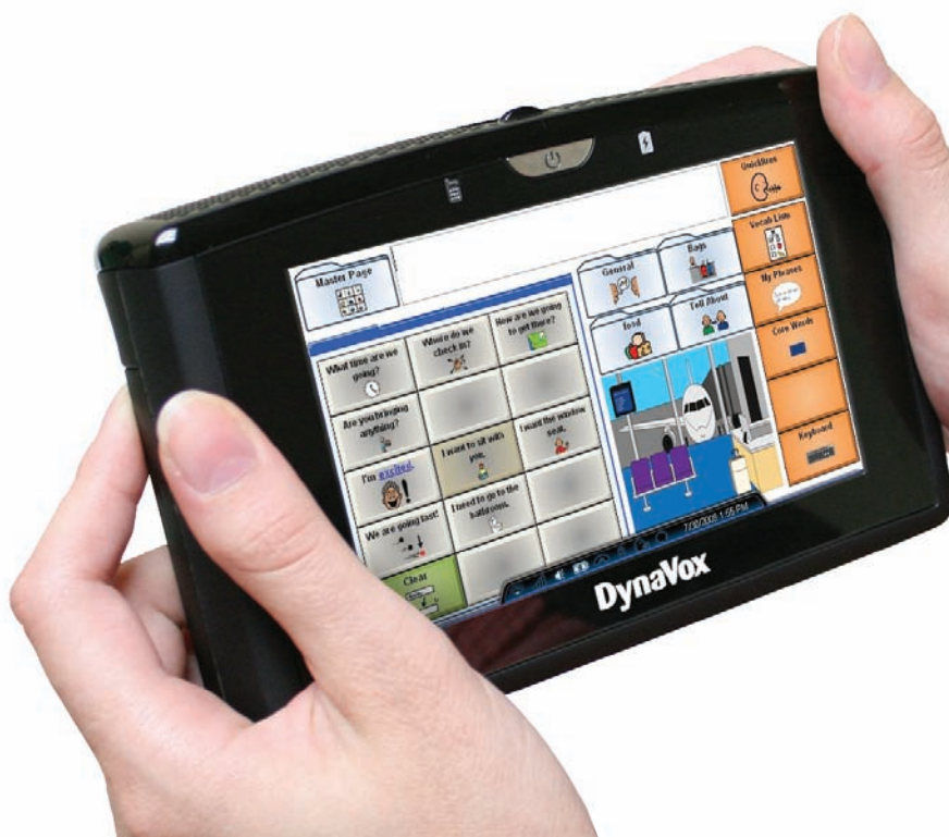
Figure 1 | DynaVox Xpress is a battery-powered speech-generating device based on technology tailored to an individual user's disabilities, age, and needs.
