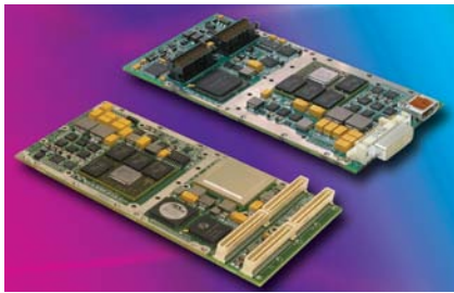
Figure 2 | Aitech's rugged M595 PMC and M597 XMC cards are used in avionics applications.
