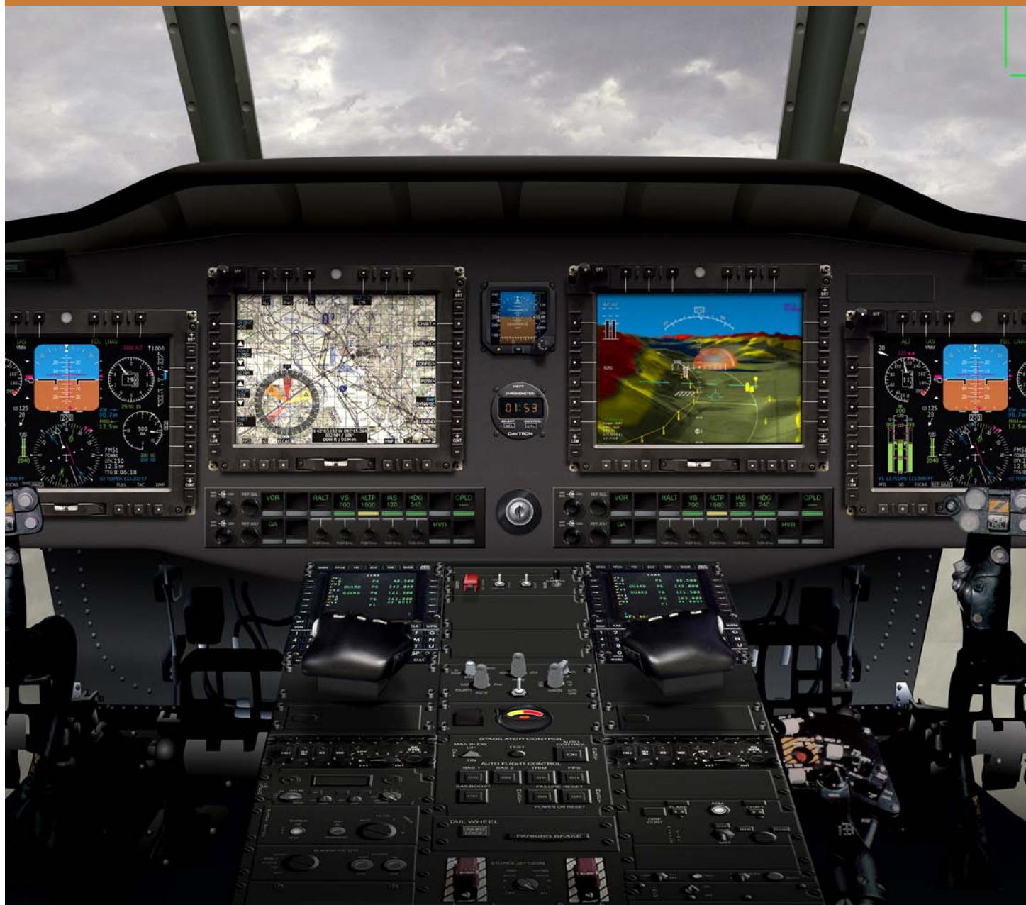
The Black Hawk UH-60M cockpit uses Rockwell Collins avionics and synthetic vision technology in the right-hand inboard multifunction display.
