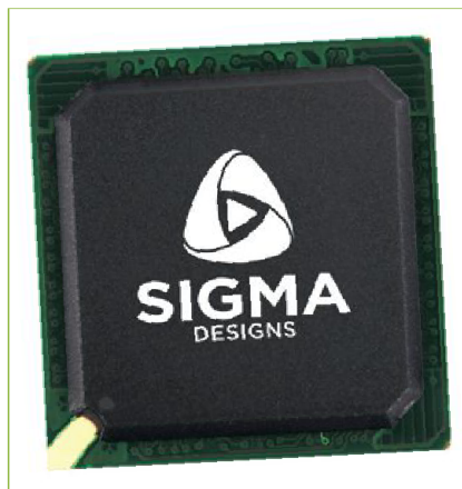
Figure 2 | Sigma Designs uses frequency scaling and power islanding techniques with its chips to achieve low power.
