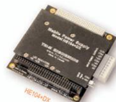
108 Watt PC/104+ Power Supply
